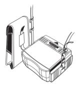
Pass the strap belt down through the side panel of the main body from the top, and up through the slots of the probe case from the bottom.
